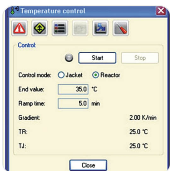
Manual operation, for example temperature control
