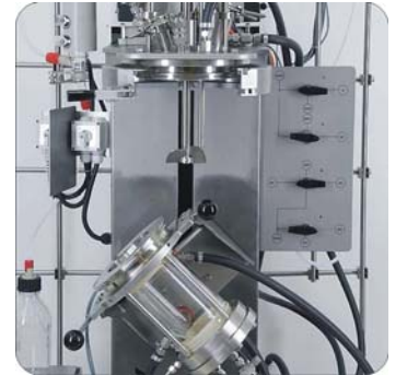
Easy loading of product into the lowered and tilted vessel
